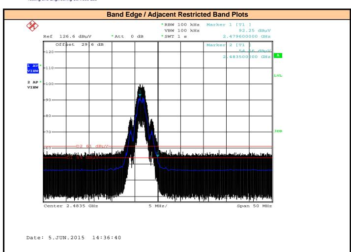
Band Edge / Adjacent Restriced Band 2483.5MHz (High Channel) - Horizontal
