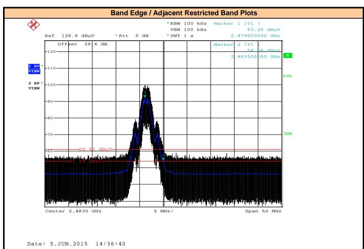
Band Edge / Adjacent Restriced Band 2483.5MHz (High Channel) - Vertical
