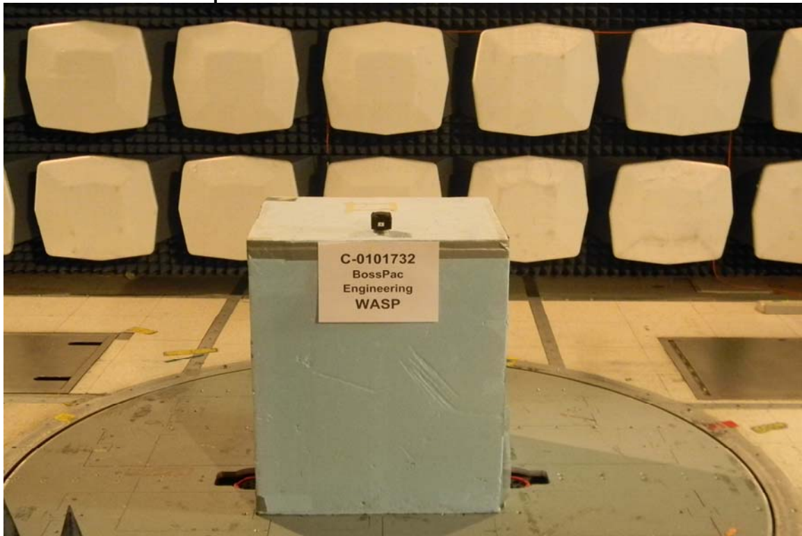
Radiated Emission setup
