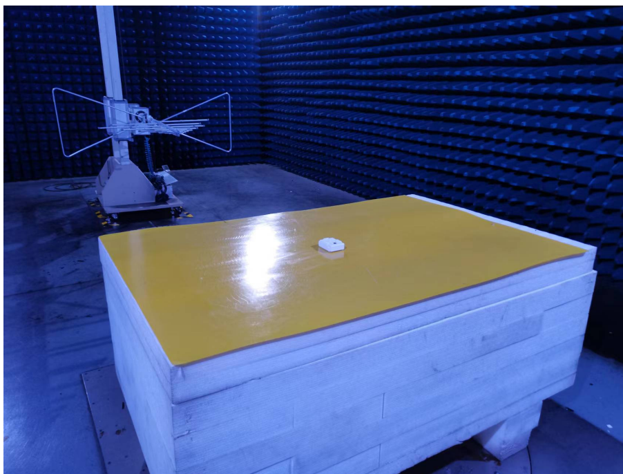
Photo of Radiated Emission Measurement (Below 1G)
