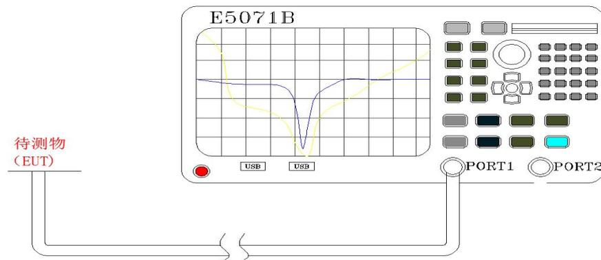
Fig.1 Antenna measured in Network Analyzer
