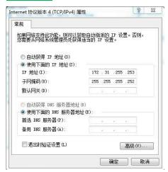
A fall back IP 172.31.255.254/255.255.255.252 is assigned to DT01's LAN port so user can always access DT01 with this ip if their laptop has the IP 172.31.255.253/255.255.255.252.
