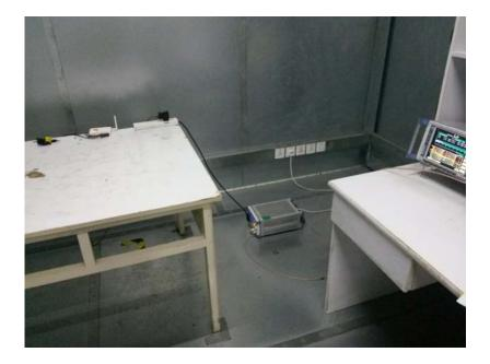
1.1. Set-up for Conducted Emission Test
