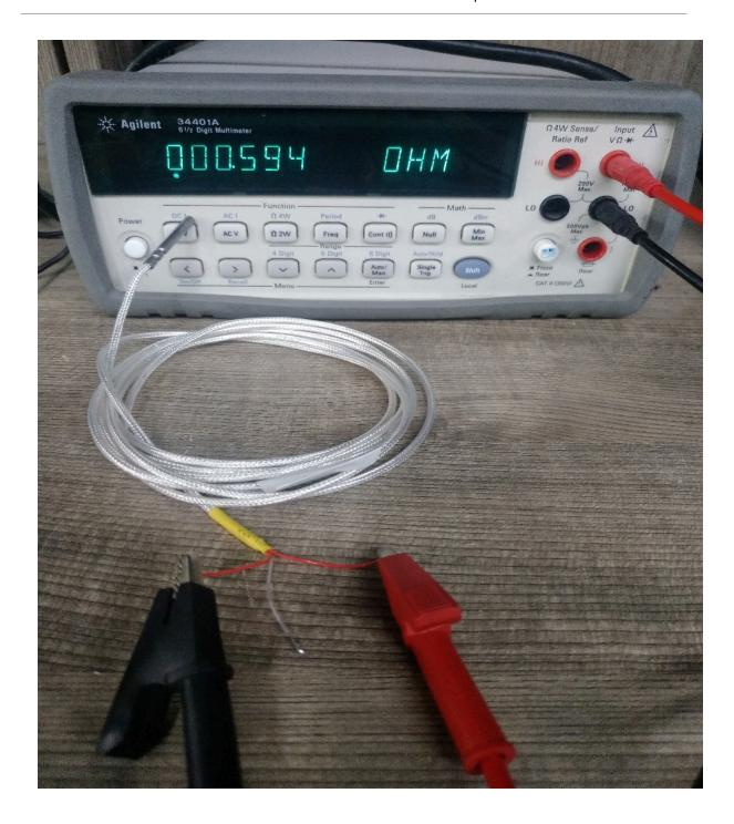
As example, in this step, we check the shorted wire (both red) with 0.594 ohm, So we know that each wire of PT100 has (0.594-0.002)/2=0.296R (Where 0.002 is the value we got from step 1) .
