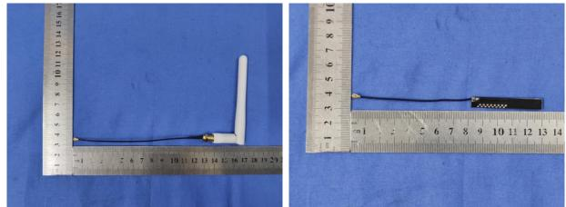
Antenna gain : 2dBi Model: AN2400-5701SM Manufacturer: Dongguan meimei electronics factory Antenna gain : 2dBi Model: NB004-113B-125IX Manufacturer: Dongguan honuo electronics co. LTD Sincerely,
