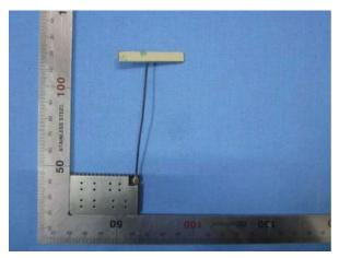
New: External Antenna with unique non standard antenna port Antenna gain: 1.5dBi
