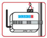
Connect the cable from the current clamp to the MS12's input port. Take care of connecting the black and red cable as shown in the drawing on the left. Only apply gentle force when fastening the two screws.
