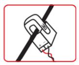
For safety reasons, switch off the main electricity supply. For a single phase supply, attach the current clamp to one of the two cables running from the electricity meter to the fuse box. Close the clamp firmly.
