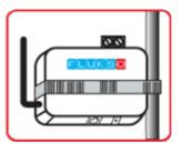
Disconnect all cables from the Fluksometer. Find a suitable location near the fuse box to install the Fluksometer. Secure the Fluksometer with the plastic cable tie.
