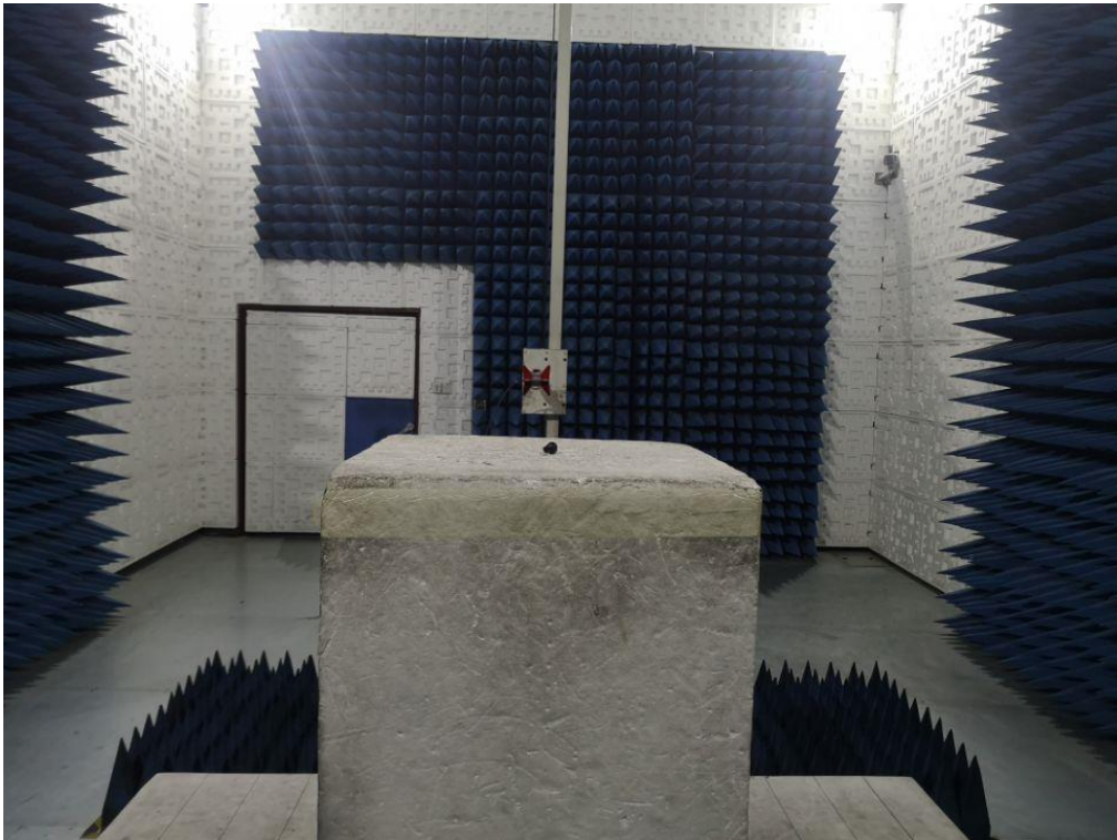
RADIATED EMISSION TEST SETUP ABOVE 1GHZ
