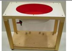
The bottom plate contains three pair of bolts for locking the device holder. The device holder positions are adjusted to the standard measurement positions in the three sections. A white cover is provided to tap the phantom during off-periods to prevent water evaporation and changes in the liquid parameters. On the phantom top, three reference markers are provided to identify the phantom position with respect to the robot.
