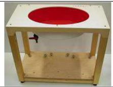
The bottom plate contains three pair of bolts for locking the device holder. The device holder positions are adjusted to the standard measurement positions in the three sections. A white cover is provided to tap the phantom during off-periods to prevent water evaporation and changes in the liquid parameters. On the phantom top, three reference markers are provided to identify the phantom position with respect to the robot.
