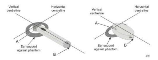
An alternative form factor DUT with reference points and reference lines
