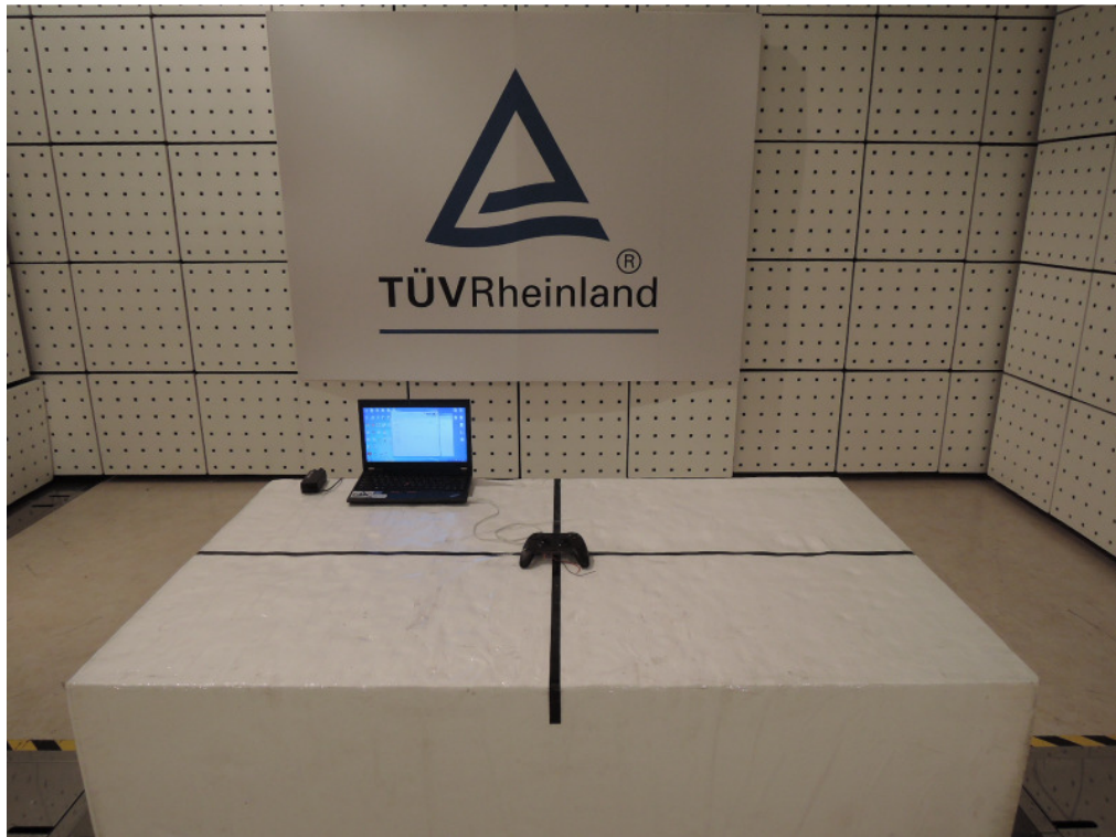
Photograph 2: Set-up for Spurious Emissions (Back View 1)
