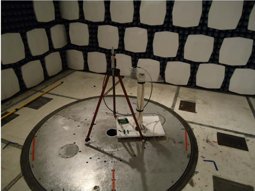
Radiated Measurements in Semi-Anechoic Chamber
