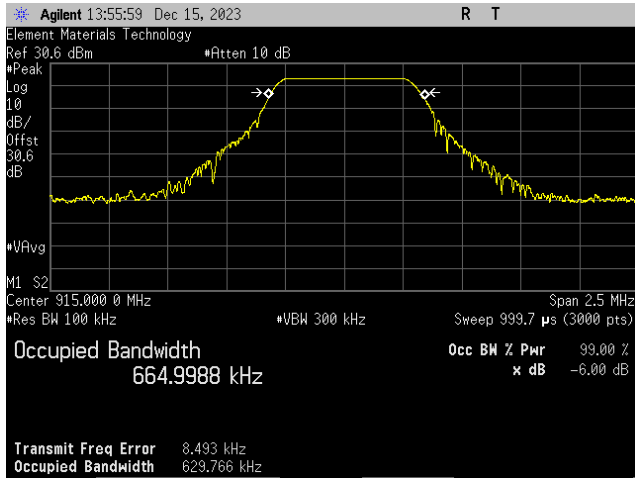
LoRa, Spreading Factor = 8, 500 kHz BW, Coding Rate =4/8 External Antenna Port Mid Ch. = 915 MHz
