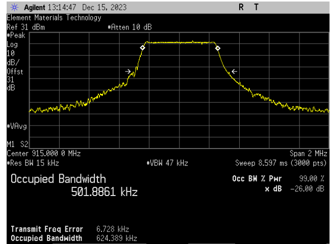
LoRa, Spreading Factor = 8, 500 kHz BW, Coding Rate =4/8 Internal Antenna Port Mid Ch. = 915 MHz
