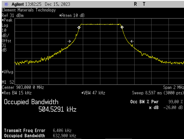
LoRa, Spreading Factor = 8, 500 kHz BW, Coding Rate =4/8 Internal Antenna Port Low Ch. = 903 MHz
