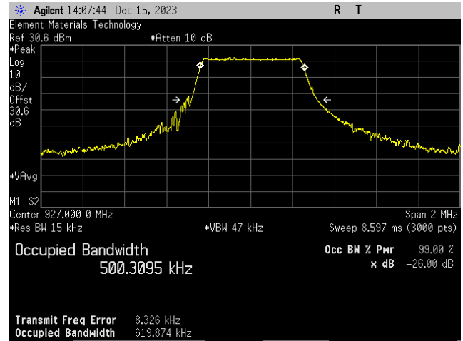
LoRa, Spreading Factor = 8, 500 kHz BW, Coding Rate =4/8 External Antenna Port High Ch = 927 MHz
