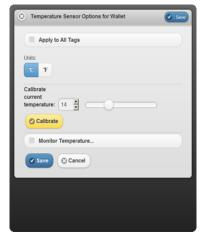
The temperature sensor often needs calibration to remove an offset. In the "Calibrate current temperature" section, set the correct current temperature, and click the "Calibrate" button.
