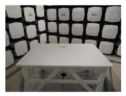
9.2 Radiated Emissions (Below 1 GHz) – Rear View
