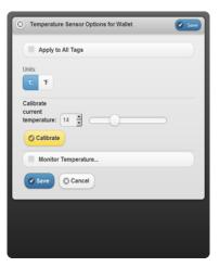
The temperature sensor often needs calibration to remove an offset. In the "Calibrate current temperature" section, set the correct current temperature, and click the "Calibrate" button.
