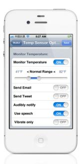
Open the temperature sensor options for each tag individually by tapping the gear icon at the bottom.
