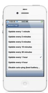
Tap the refresh icon at the bottom of tag list screen, and choose any of the "Update every ..." options. Longer interval results in longer battery life but longer the out-of-range notification delay, and vice versa.
