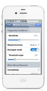
When door/gate mode is enabled, you can choose the threshold angle, when tag orientation changes more than this, the door is deemed open, when tag orientation returns within this threshold, it is deemed closed.
