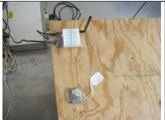
Conducted Emission Test setup - Rear
