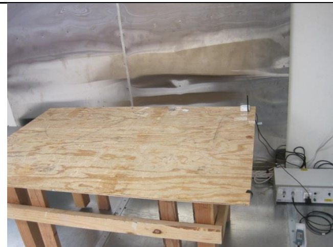
Conducted Emission Test setup - Front
