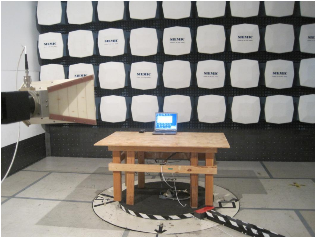
Radiated Emission (1GHz - 5GHz) – Front View
