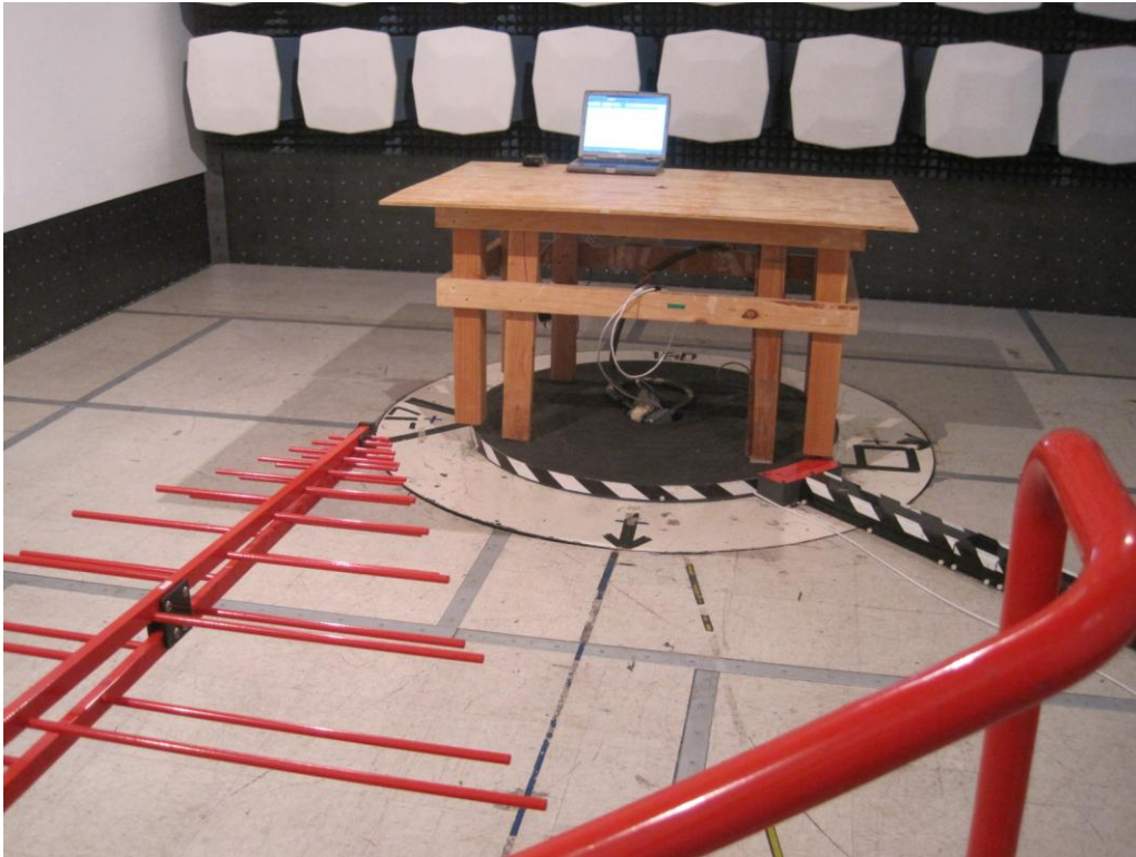
Radiated Emission (30 MHz – 1GHz) – Front View
