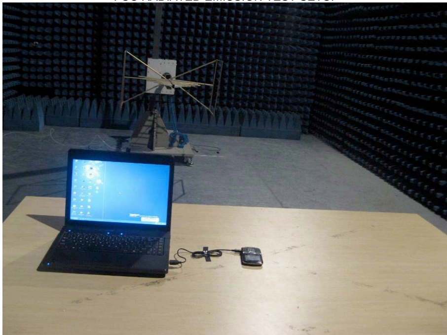
FCC RADIATED EMISSION TEST SETUP
