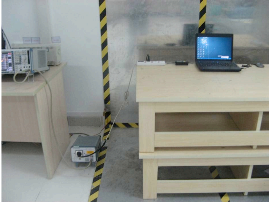
FCC LINE CONDUCTED EMISSION TEST SETUP
