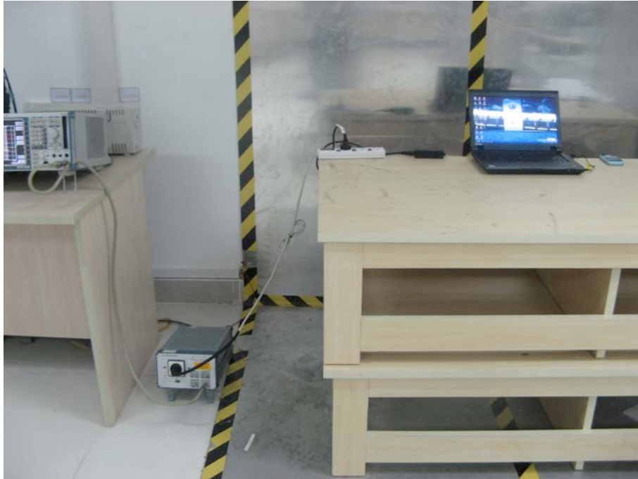
FCC LINE CONDUCTED EMISSION TEST SETUP
