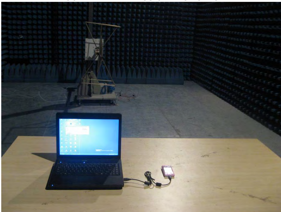
FCC RADIATED EMISSION TEST SETUP
