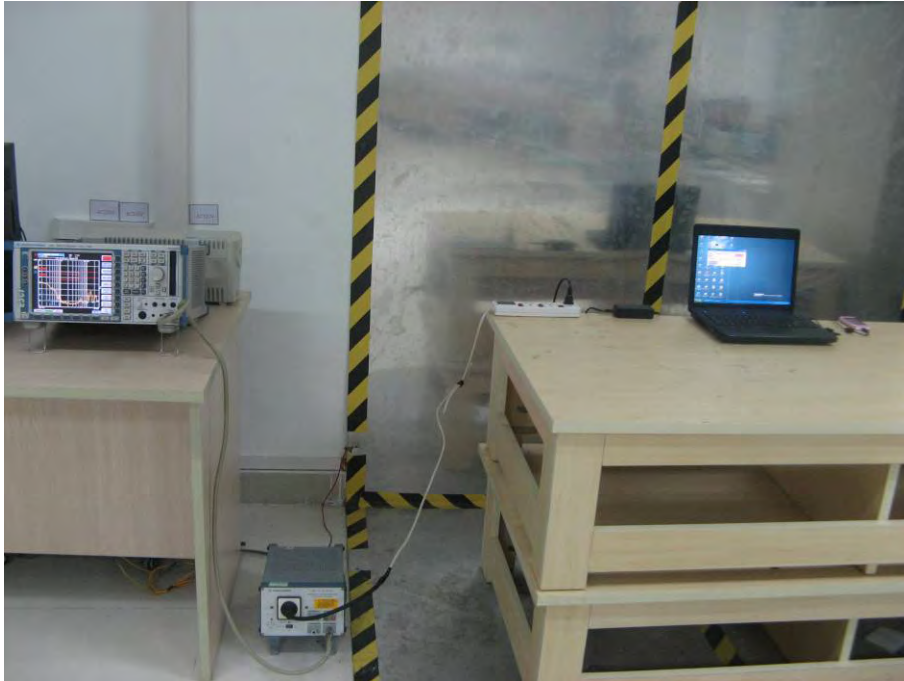
FCC RADIATED EMISSION TEST SETUP
