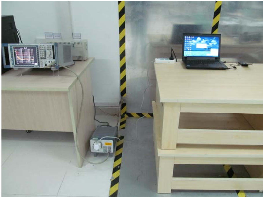
FCC RADIATED EMISSION TEST SETUP
