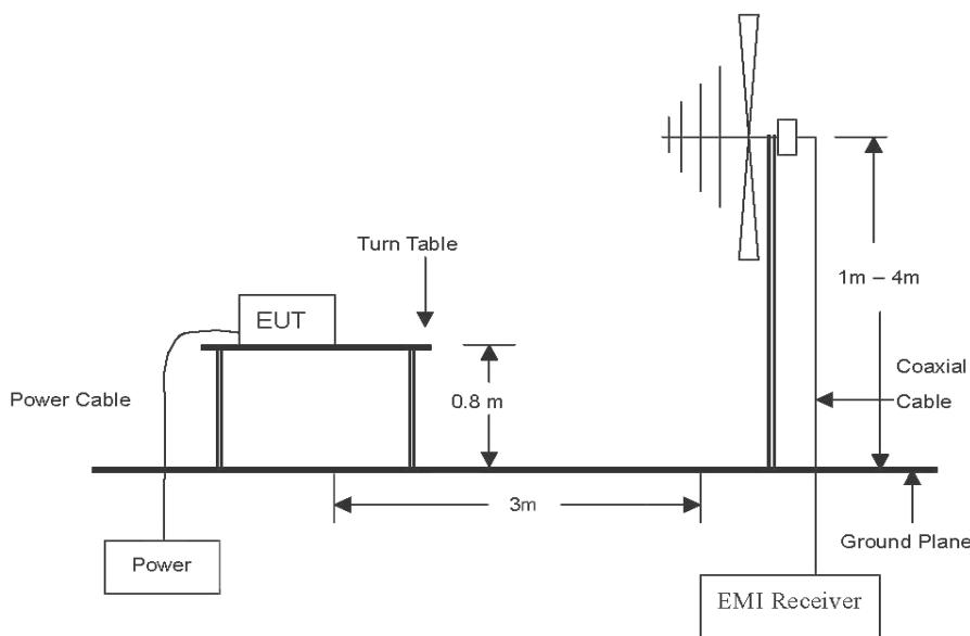
The diagram below shows the test setup that is utilized to make the measurements for emission from 1 GHz to 24 GHz emissions.
