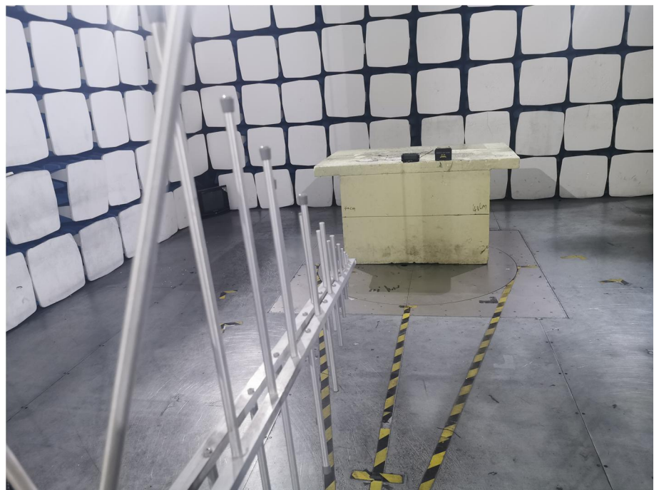
Radiation Emission Test Setup (30MHz to 1GHz)
