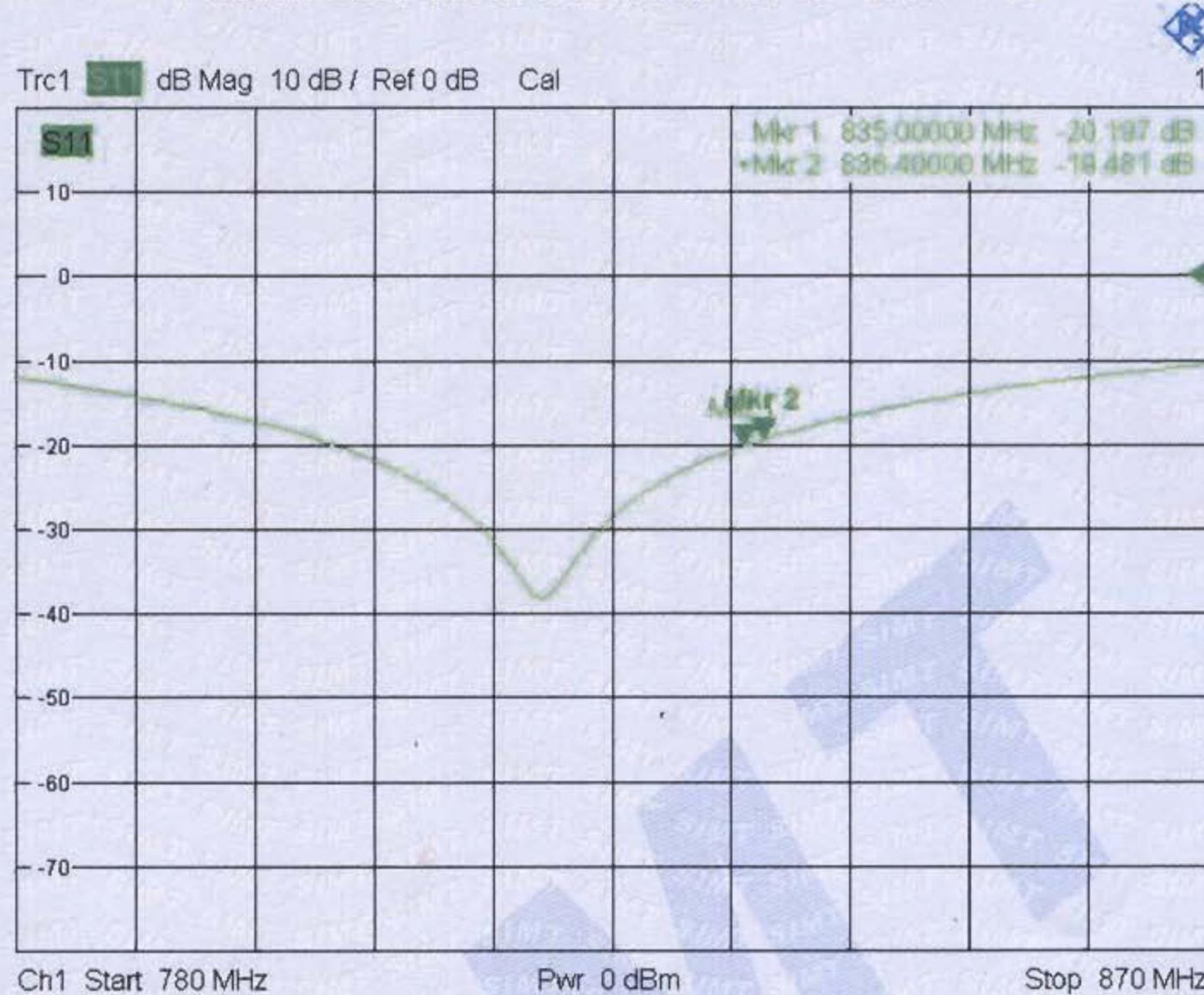
**Return Loss Measurement Plot for Body TSL**
