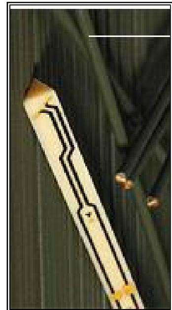
Inside View of SN11/09 EP100 E-field Probe
