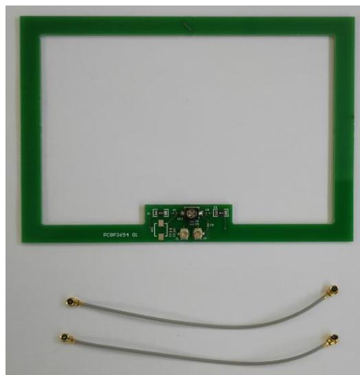
**NOTE:** The Antenna and the U.FL coax cables can be supplied by Access IS or the user can design the antenna using the support provided by Access IS. U.FL cables are widely available from electronics stores like RS/Farnell.
