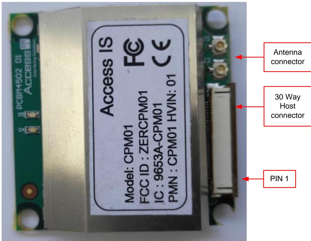
The following table shows the pinouts for the host connector.
