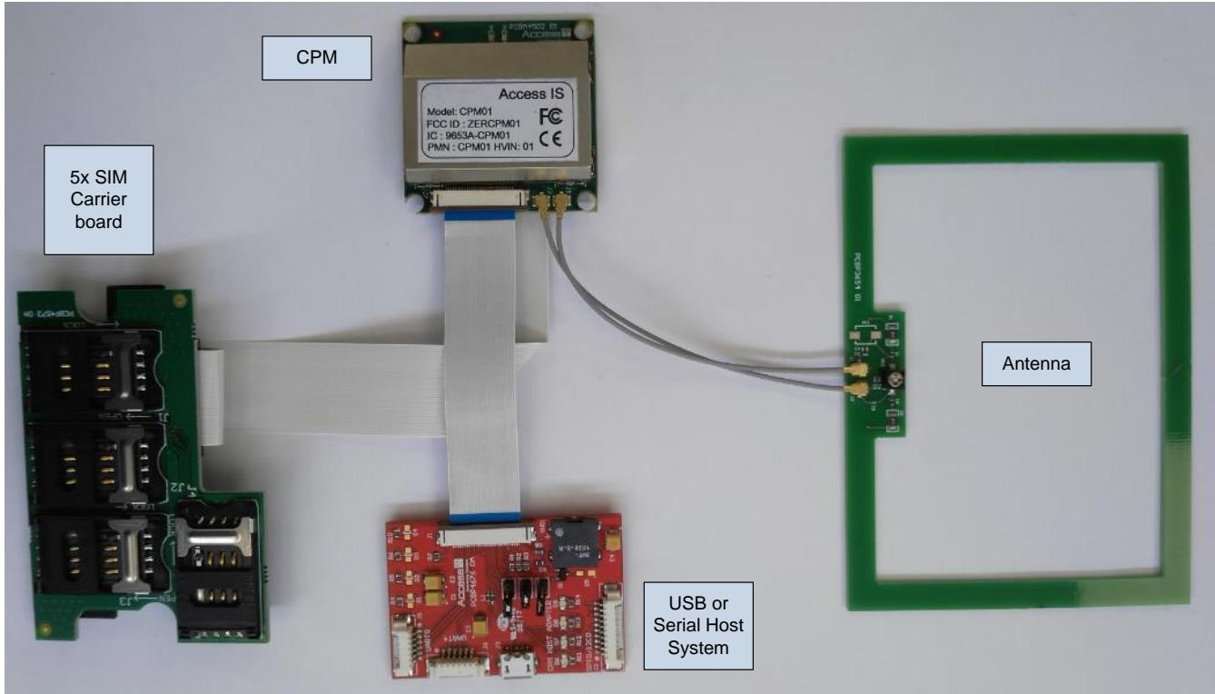
5, After the connections are done, select/verify the correct host interface selection on HOST\_IFSEL\_IO pins.
