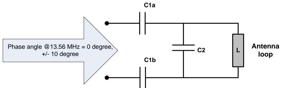
The Antenna is tuned to resonate at 13.56MHz with a phase angle tolerance of +/-10 degrees. The following graph shows the impedance and phase for a typical antenna tuned to 13.56MHz.
