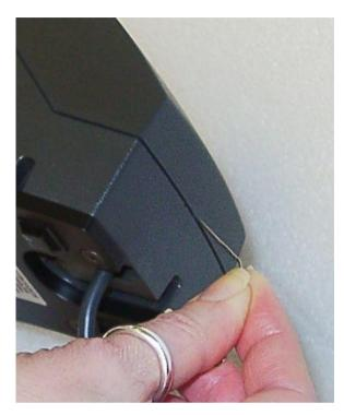
The BGR135 connects by means of an RJ-50 10-pin modular socket on the back of the unit.
