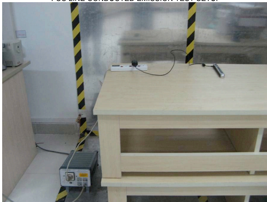
FCC LINE CONDUCTED EMISSION TEST SETUP
