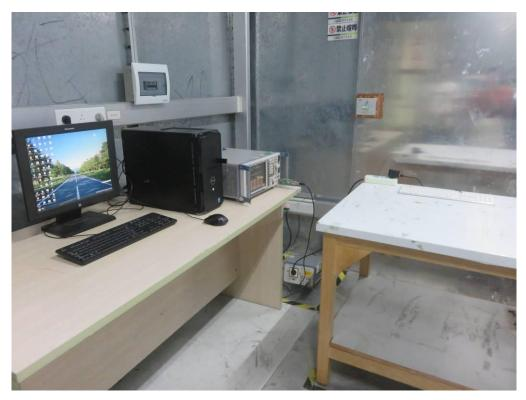
FCC RADIATED EMISSION TEST SETUP
