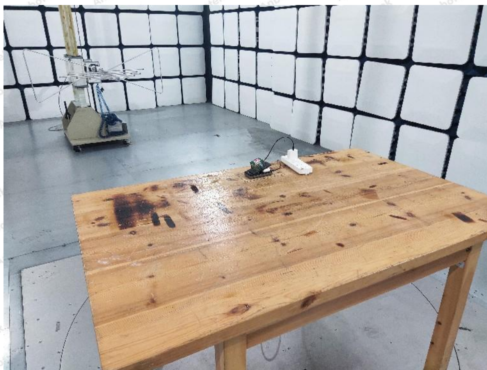
Photo of Radiation Emission Test
