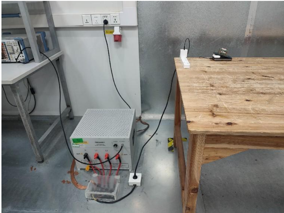
FCC ID:ZE9-ST-UCDWPBSM Photo of Conducted Emission Measurement
