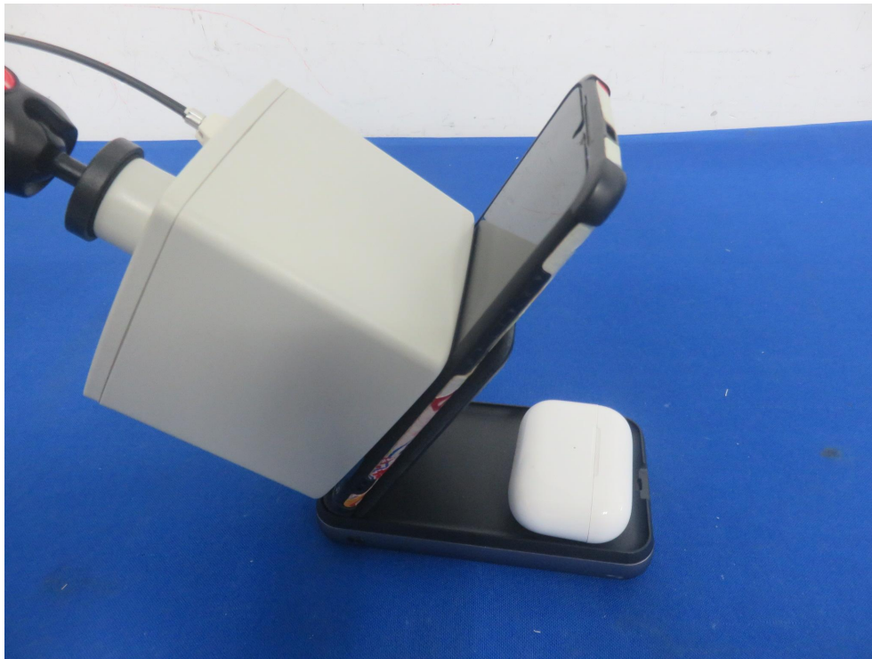
Photo of MPE Measurement at 0 cm
