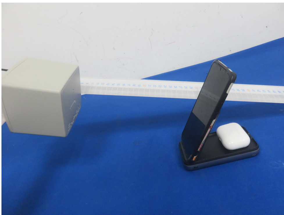
Photo of MPE Measurement at 20 cm
