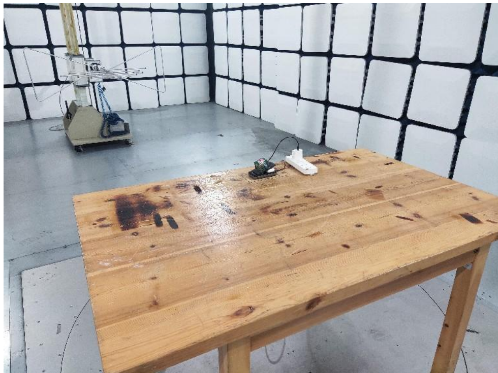
Photo of Radiation Emission Test
