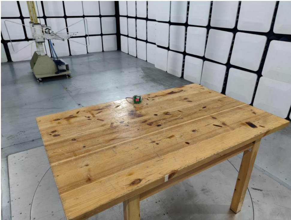
FCC ID: ZE9-ST-MCMWCM Photo of Radiation Emission Test
