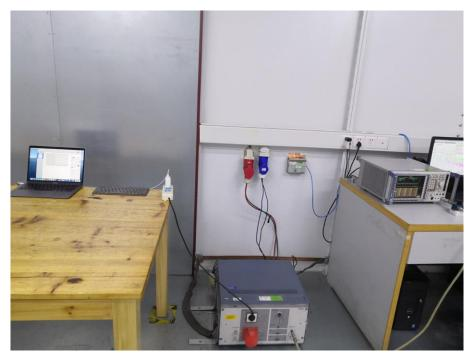
FCC RADIATED EMISSION TEST SETUP
