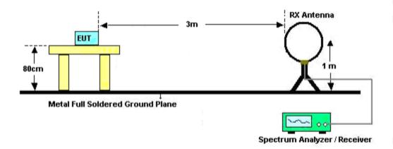
(B) Radiated Emission Test-Up Frequency 30MHz~1GHz
