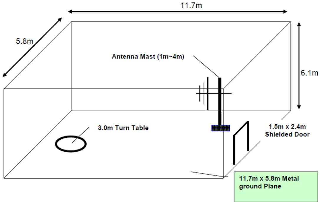
**FIGURE 1 - LAYOUT OF 3 METER SEMI-ANECHOIC CHAMBER**
