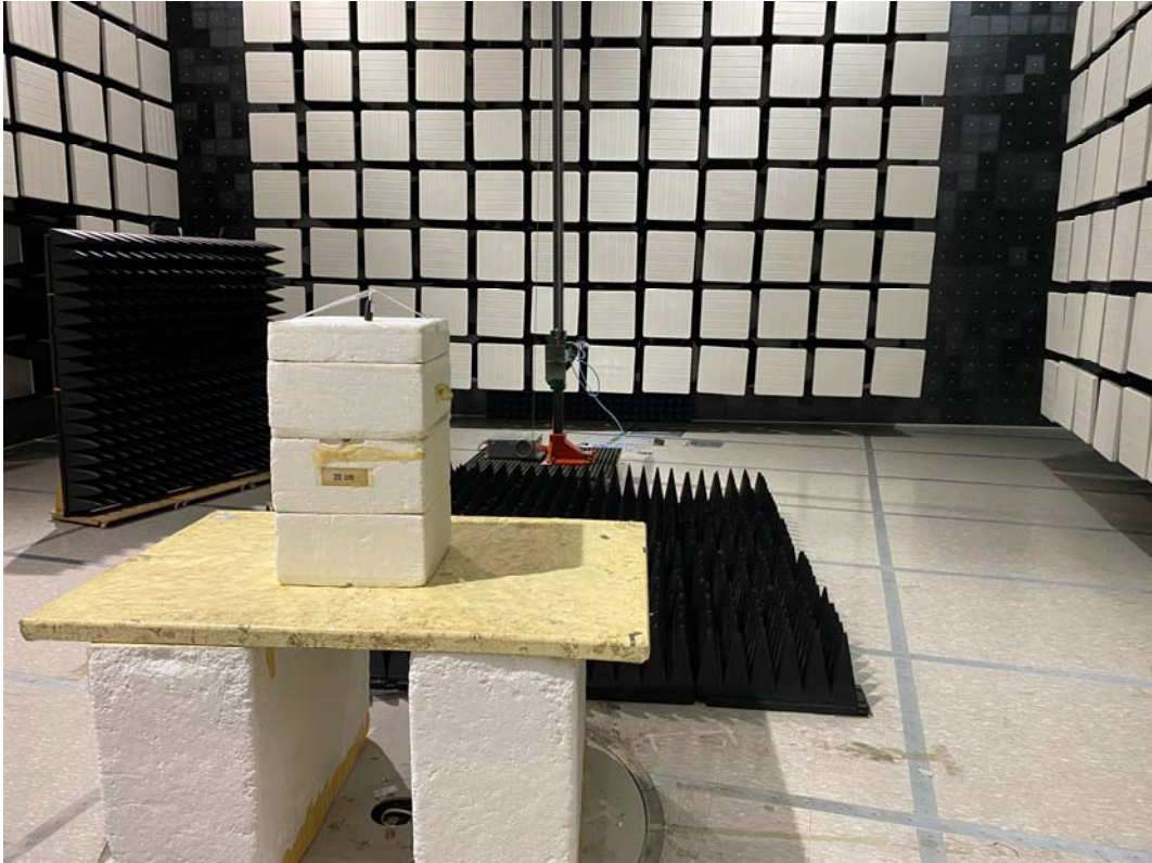
Radiated emission test (1 GHz to 5 GHz) – Front view
