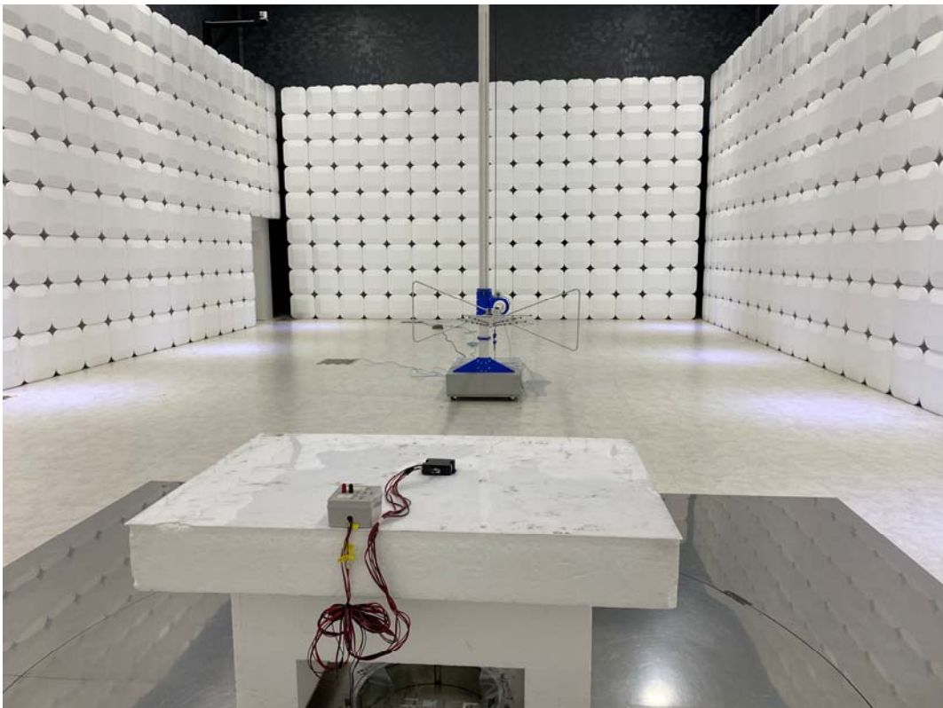
Radiated emission test (30 MHz to 1 GHz) – Rear view
