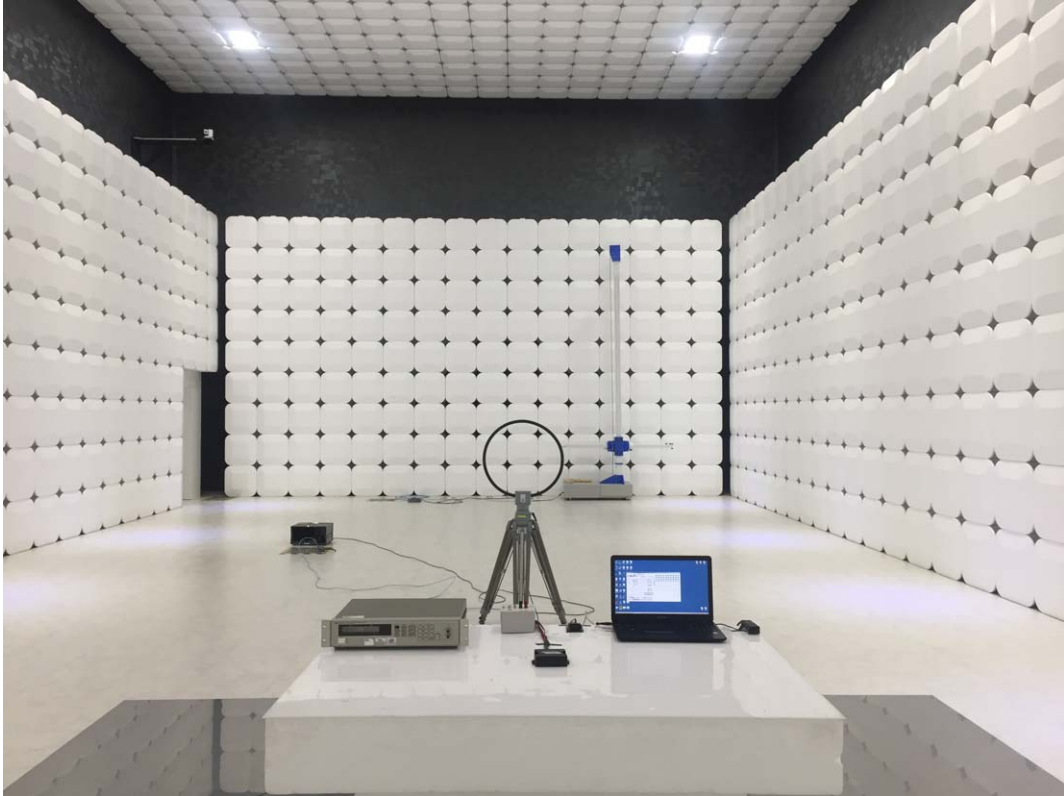
Radiated emission test (9 kHz to 30 MHz) – front view
