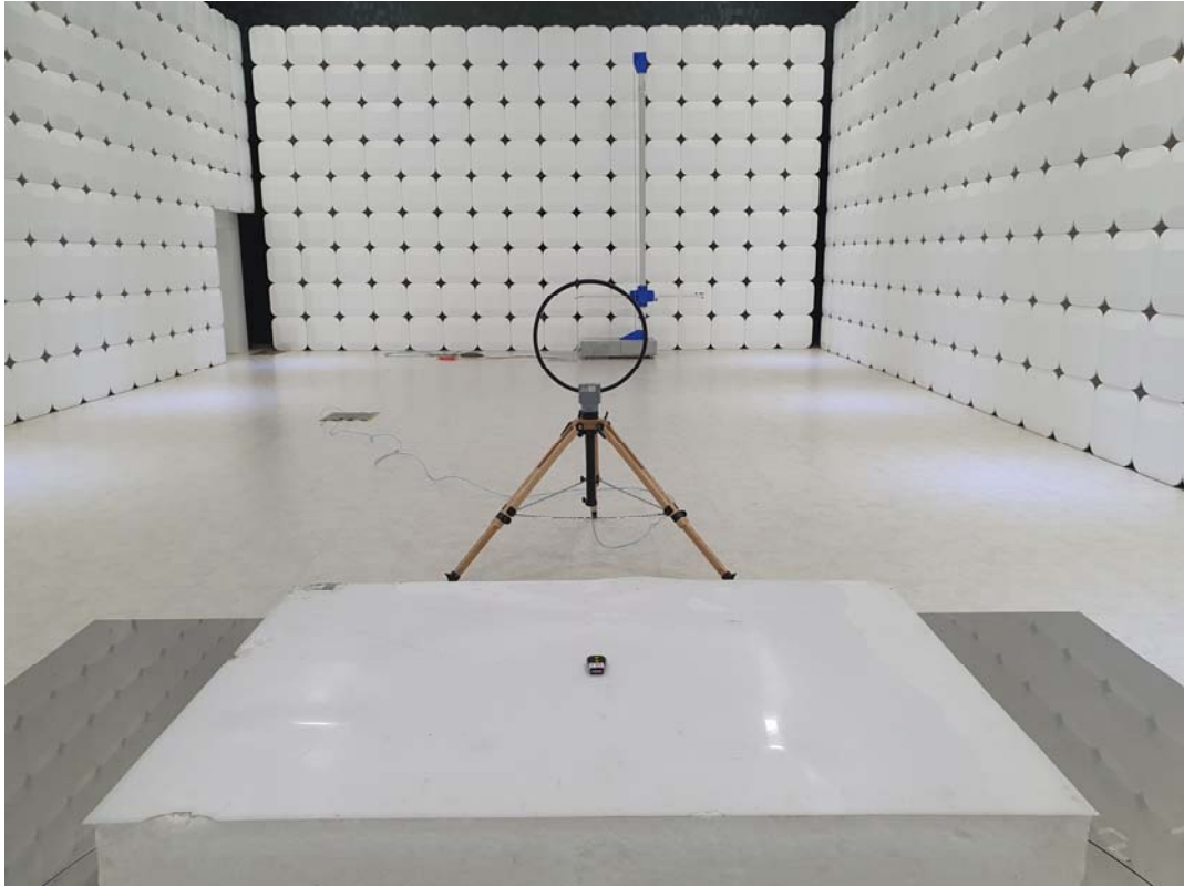
Radiated emission test (9 kHz to 30 MHz)
