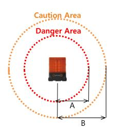
Figure 2. IPAS Flash Light Tag Detecting Distances
