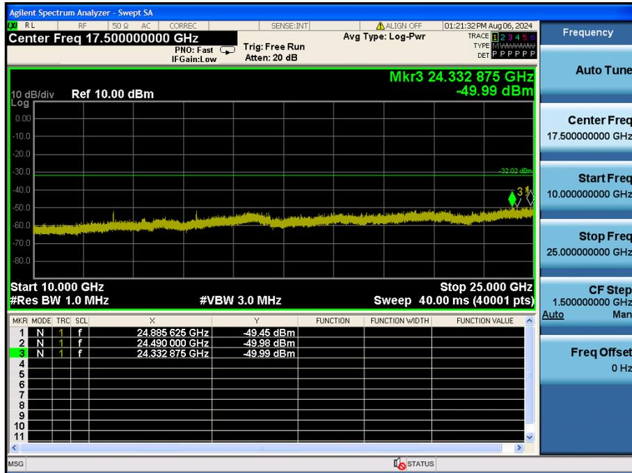
TM 1 Conducted Spurious Emissions – Zoom Plot 1 (Test Channel : Highest)
