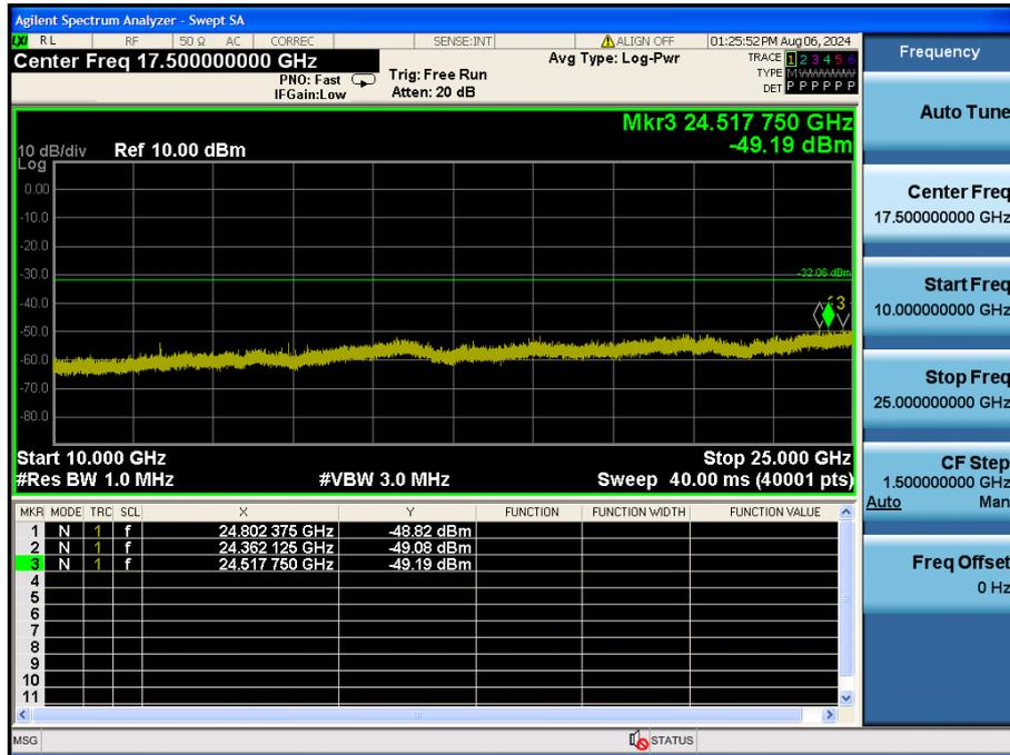
TM 2 Conducted Spurious Emissions – Zoom Plot 1 (Test Channel : Lowest)
