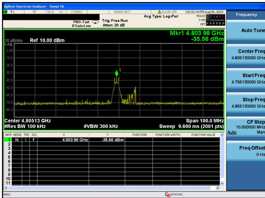
TM 2 Conducted Spurious Emissions – Zoom Plot 2 (Test Channel : Lowest)
