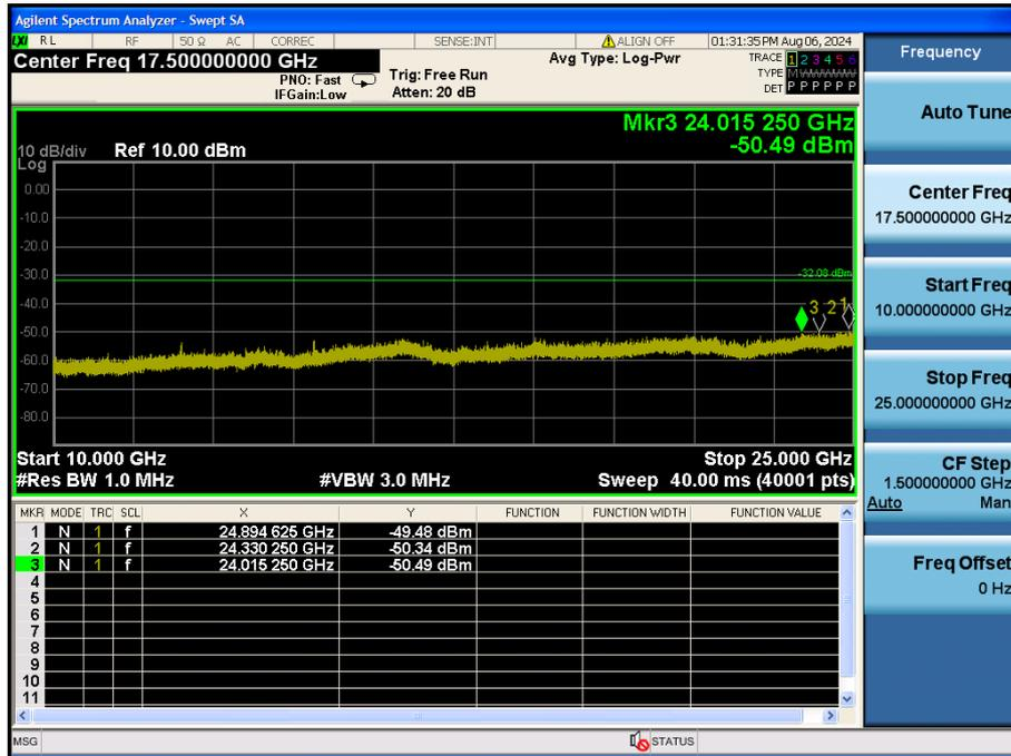
TM 2 Conducted Spurious Emissions – Zoom Plot 1 (Test Channel : Highest)
