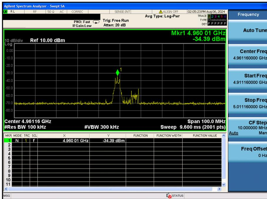
TM 2 Conducted Spurious Emissions – Zoom Plot 2 (Test Channel : Highest)
