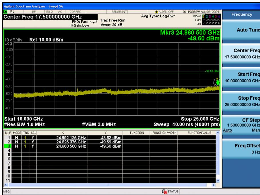
TM 1 Conducted Spurious Emissions – Zoom Plot 1 (Test Channel : Middle)
