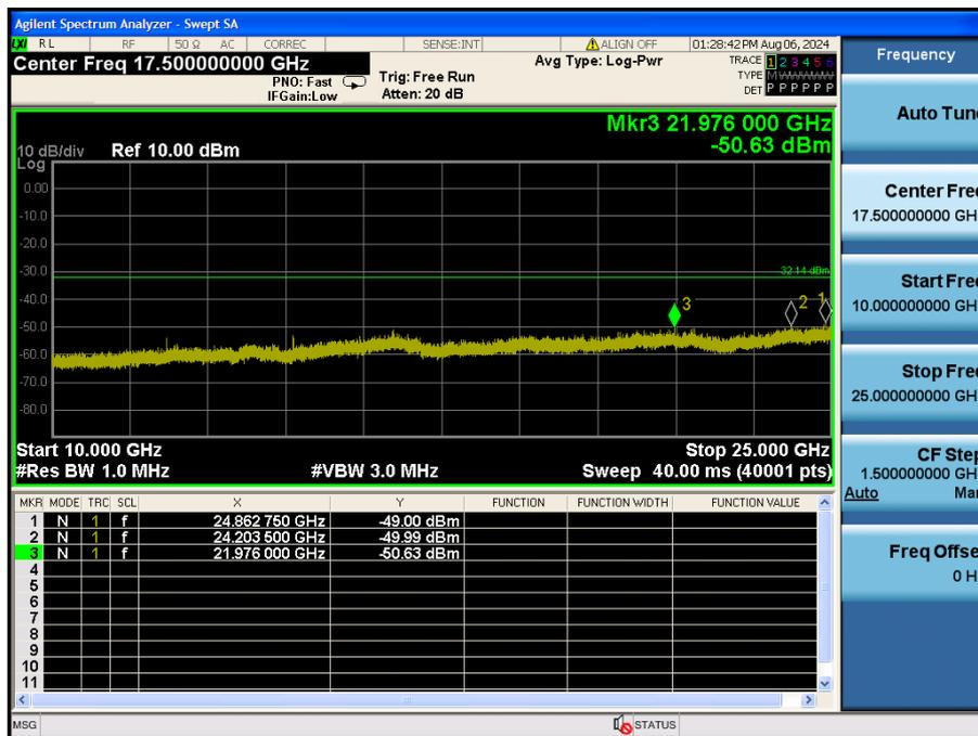
TM 2 Conducted Spurious Emissions – Zoom Plot 1 (Test Channel : Middle)
