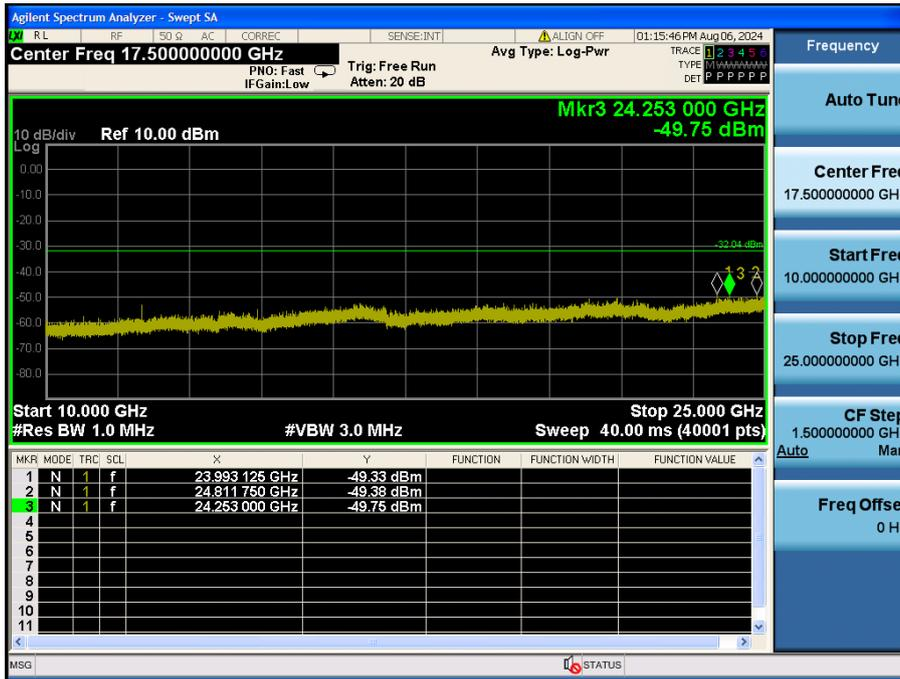
TM 1 Conducted Spurious Emissions – Zoom Plot 1 (Test Channel : Lowest)
