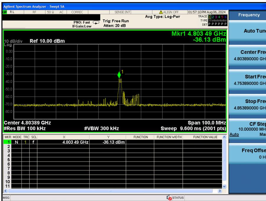
TM 1 Conducted Spurious Emissions – Zoom Plot 2 (Test Channel : Lowest)
