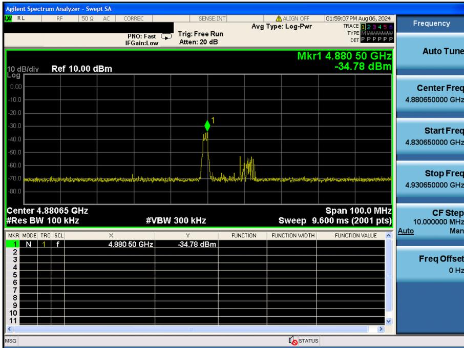
TM 1 Conducted Spurious Emissions – Zoom Plot 2 (Test Channel : Middle)
