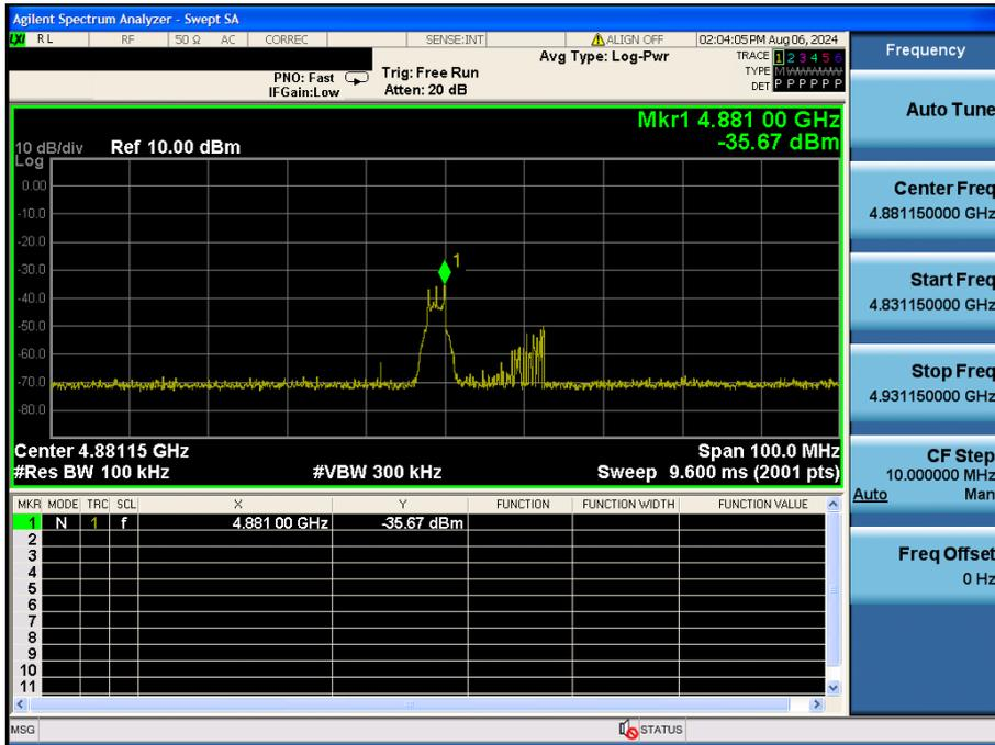
TM 2 Conducted Spurious Emissions – Zoom Plot 2 (Test Channel : Middle)
