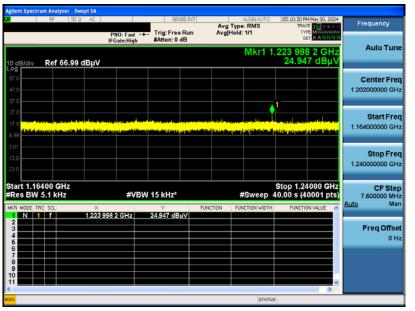
Unwanted emissions in 1 559 – 1 610 MHz Measured Level(Noise floor)
