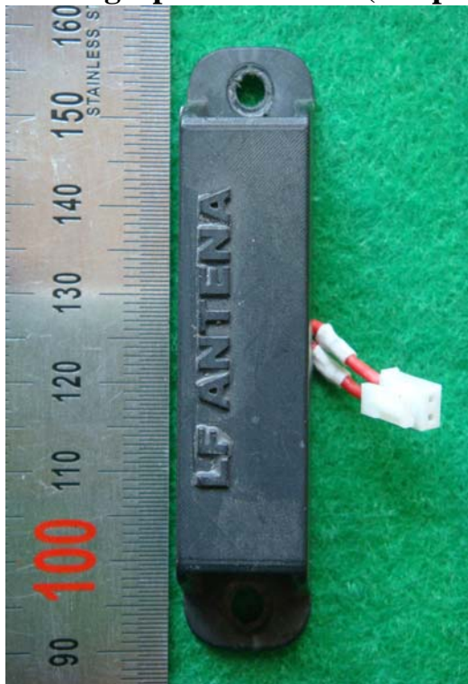
<Photograph 7: Antenna (Loop Coil antenna for 125 kHz Transmitter)>
