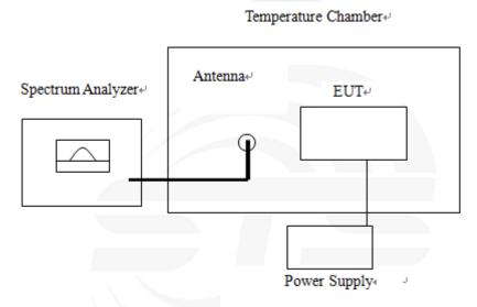
The EUT which is powered by the Battery, is coupled to the Spectrum Analyzer; the RF load attached to the EUT antenna terminal is 500hm; the path loss as the factor is calibrated to correct the reading.
