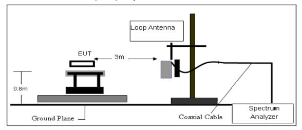
(B) Radiated Emission Test-Up Frequency 30MHz~1GHz
