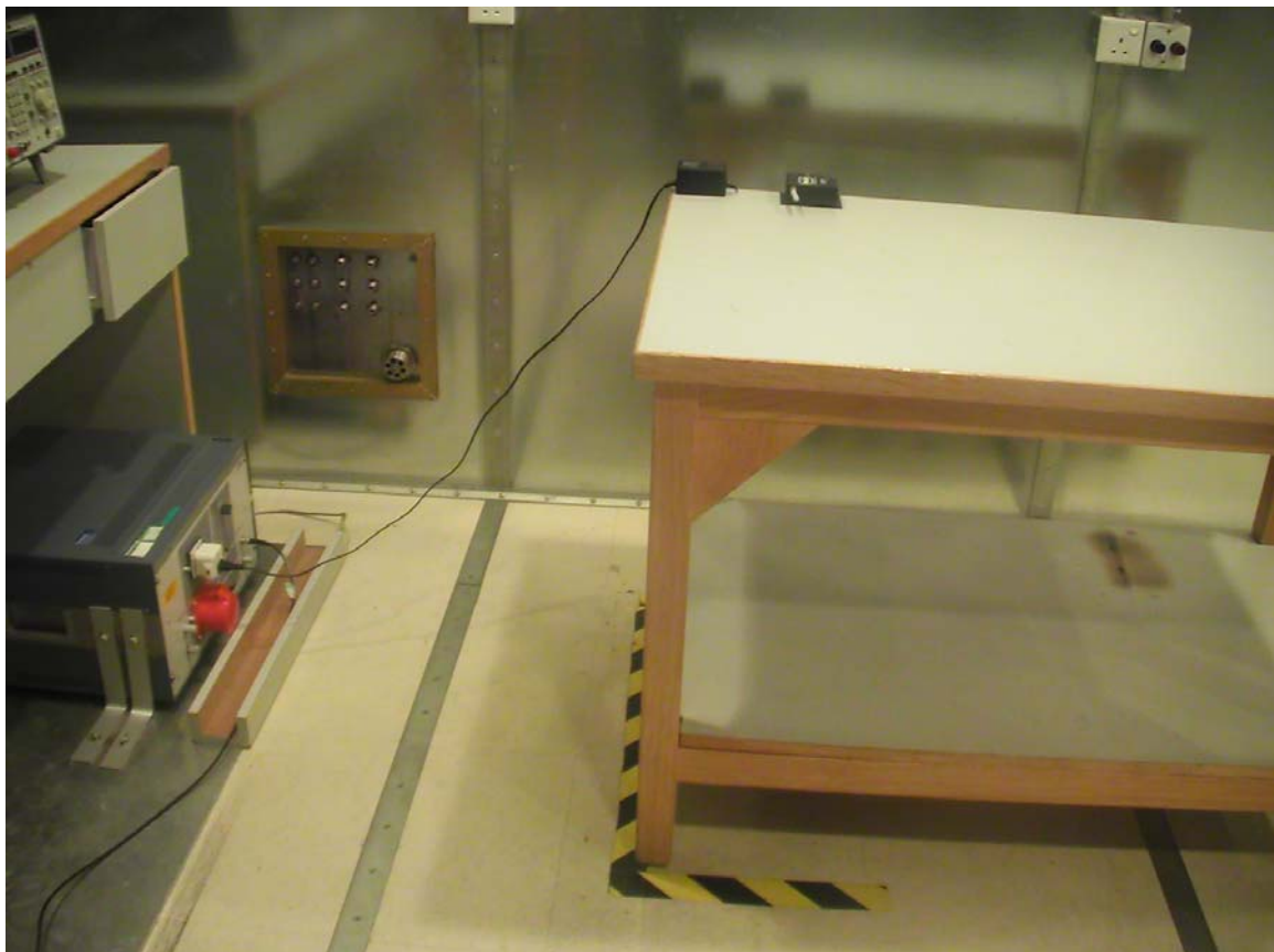
Conducted emissions test
